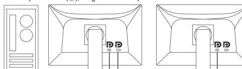
From the output terminal ( $[ \stackrel{\textbf{D}}{\tiny{\tiny B}} )$ , a signal can be output to a different monitor.
