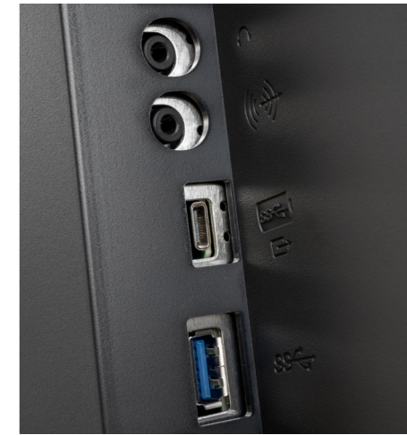
Additional USB ports and the two 3.5 millimetre sockets are installed on the side of the monitor for easier access.
