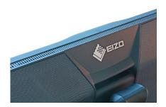
Rear of the EIZO CG2700X with the perforated plate
