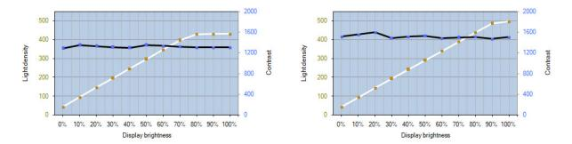
*Brightness and contrast curve of the EIZO CG2700X - D65 (DUE: Uniformity) Brightness and contrast curve of the EIZO CG2700X - D65 (DUE: Brightness)*
